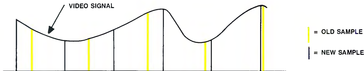
Figure 4. Filters interpolate value for new samples on a horizontal TV line. The new samples are in the correct position for the destination format's line length.
